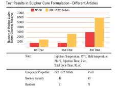
Test Results in Sulphur Cure Formulation (EPDM 100, oil 90, CB 140, curative 3.5, processing aid 3.5 phr)
