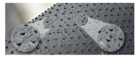
Effect of O<sub>3</sub> on unprotected rubber Effect of O<sub>2</sub> on unprotected rubber Note: The orientation of the cracks on the surface of the rubber. Photo courtesy of Akron Rubber Development Lab
